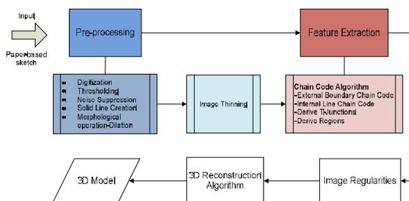
Fig. 3: Methodology of 3D reconstruction from paper sketches
