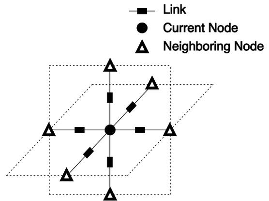
Fig. 1. Link interconnection between nodes in proposed network. Only a single spring is embedded for each link.
