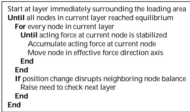
Fig. 3. Steps to distribute resulting force from loading area to the surrounding node network.
