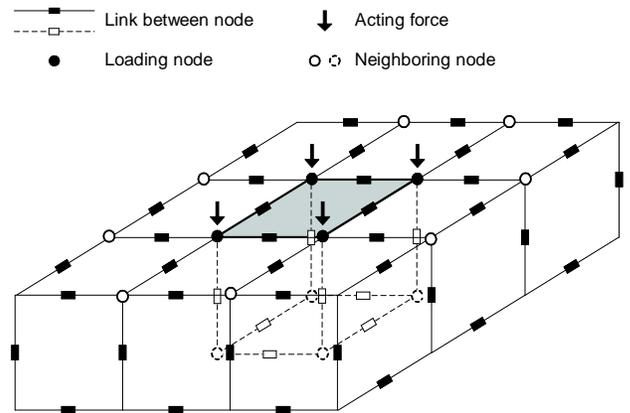
Fig. 4. Working node network. Loading area is colored with gray shade which is imposed with external acting force depicted with arrows.
