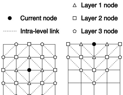
Fig. 2. Layering in node network starting from current node using top and cross-section views.
