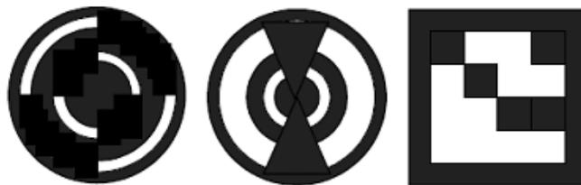
Fig. 1. Circular bar-coded markers. Taken from [10]
